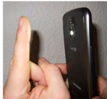
Fig. 1: Capture of the finger with the smartphone camera
