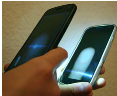
Fig. 14: Replay attack with a video on another smartphone
