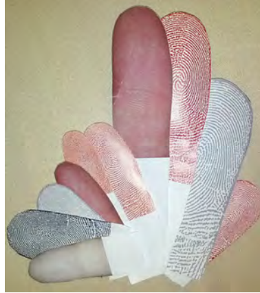
Fig. 12: Variety of tested fake 2D print outs
