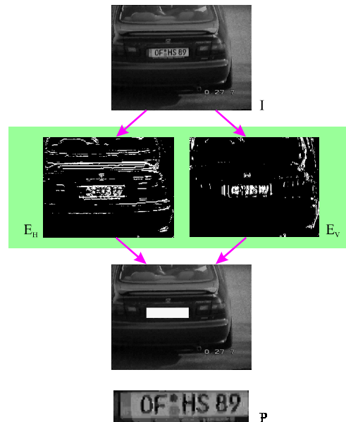
Fig. 5: Edge based license plate segmentation
