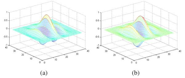
Figure 1. One complex Gabor filter ( $f = 0.1, \sigma_x = 6.0, \sigma_y = 6.0, \theta = 1/2\pi$ ). (a) the real part of the complex Gabor filter; (b) the imaginary part of the complex Gabor filter.
