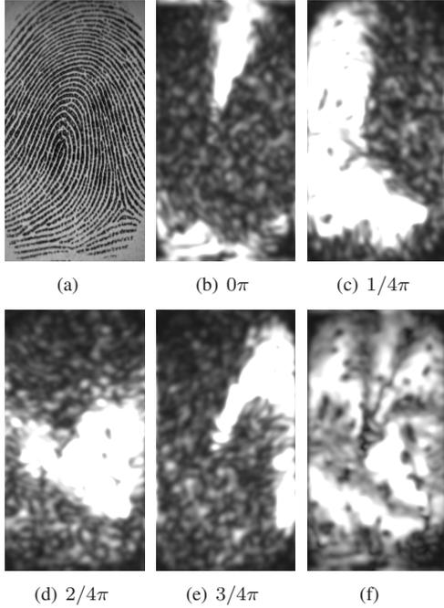
Figure 2. Fingerprint from FVC2002Db2 dataset and its Gabor filter responses. (a) fingerprint image; (b-e) Smoothed absolute value of fingerprint image that have been filtered by Gabor filters with different orientations; (f) the standard deviation value of Gabor responses with different orientations.
