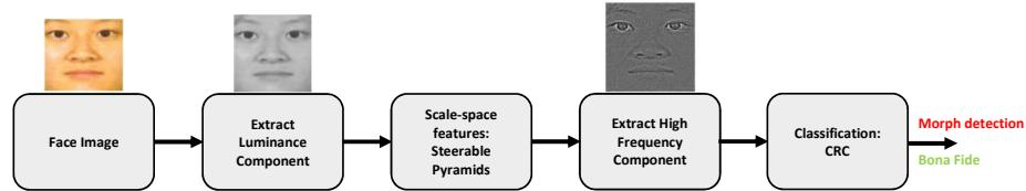
Fig. 1: Block Diagram of the Proposed Method
