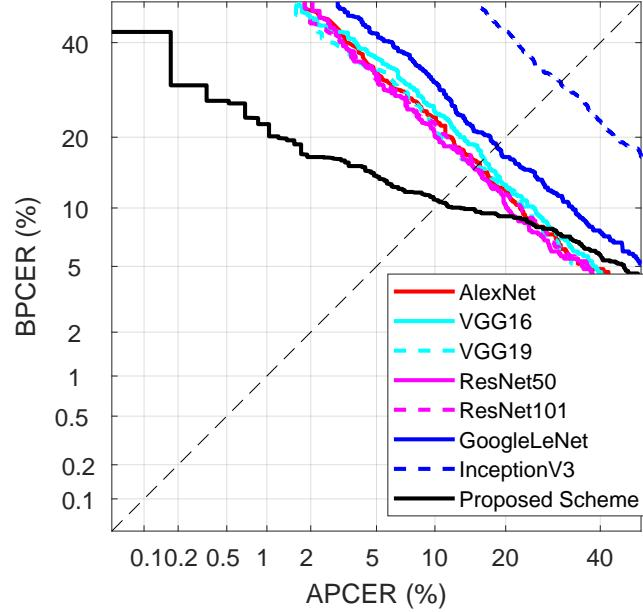
Fig. 5: DET curves indicating the performance of the proposed method with Deep learning methods
