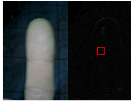
Figure 4: Blurred fingerphoto (left) and the belonging edge image (right); only the few pixel in the center (within the marked rectangle) are analyzed.
